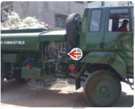
Fuel Metering System on Bouzer Ashok Leyland Chasis Export to South America
